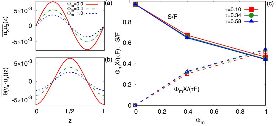
FIG. 6. Momentum budget. Mean profile (a) of the Reynolds stress term and (b) of the momentum exchange term for different mass loadings as in label, with  $\tau = 0.58$ . (c) shows the momentum budget for the amplitudes divided into Reynolds stress term (filled symbols) and exchange term (empty symbols), as a function of the mass loading  $\Phi_m$  for different values of Stokes times as in label.
