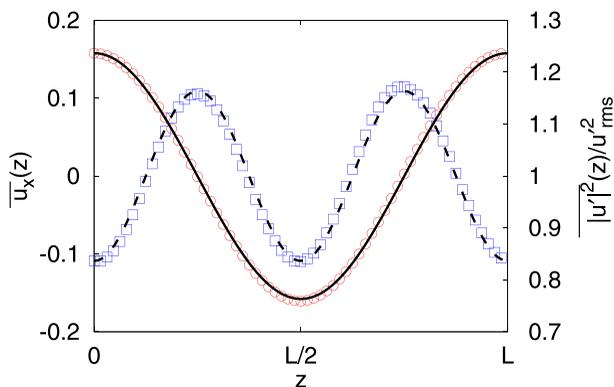
FIG. 3. Profiles of the mean longitudinal flow  $\bar{u}_x(z)$  (red circles and solid line) and the square velocity fluctuations  $\overline{|\mathbf{u}'|^2}(z)$  (blue squares and dashed line), for a simulation of the particle-laden flow with  $\tau = 0.1$ ,  $\Phi_m = 1.0$  (symbols) and a simulation of a pure fluid with rescaled forcing amplitude  $F' = F/(1 + \Phi_m)$  (black lines, data from Ref. [44]).
