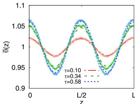
FIG. 8. Mean particle density profile  $\bar{\theta}(z)$  for different values of Stokes time (see legend) obtained with the fully Eulerian scheme with  $\Phi_m = 0.0$  (dashed curves) and with the one-way coupling Lagrangian scheme of Ref. [39] (symbols). Lagrangian data have a poorer statistics with respect to Eulerian ones, therefore to decrease a bit the statistical fluctuations we exploited the symmetry with respect to  $L/2$  to further average the density profile.
