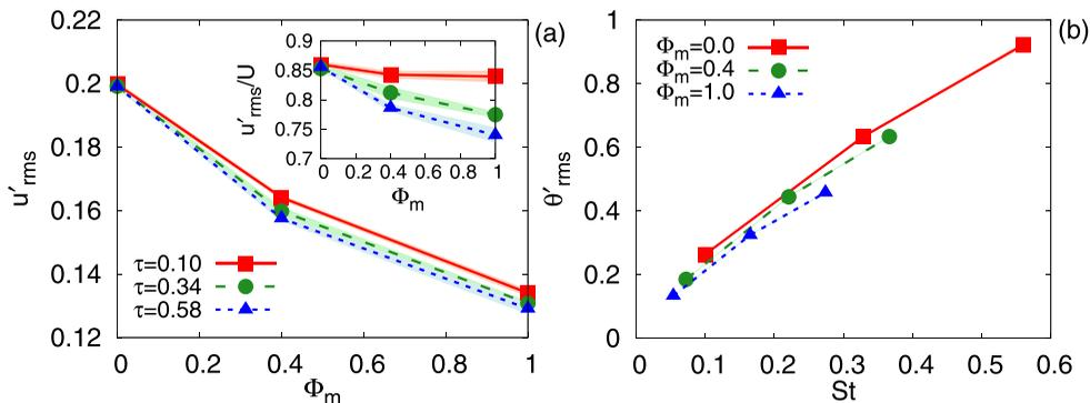
FIG. 4. (a) RMS fluid velocity fluctuations  $u'_{\text{rms}}$  as a function of  $\Phi_m$ . In the inset velocity fluctuations are normalized with the mean flow. (b) RMS particle density fluctuations  $\theta'_{\text{rms}}$  as a function of  $St$ .
