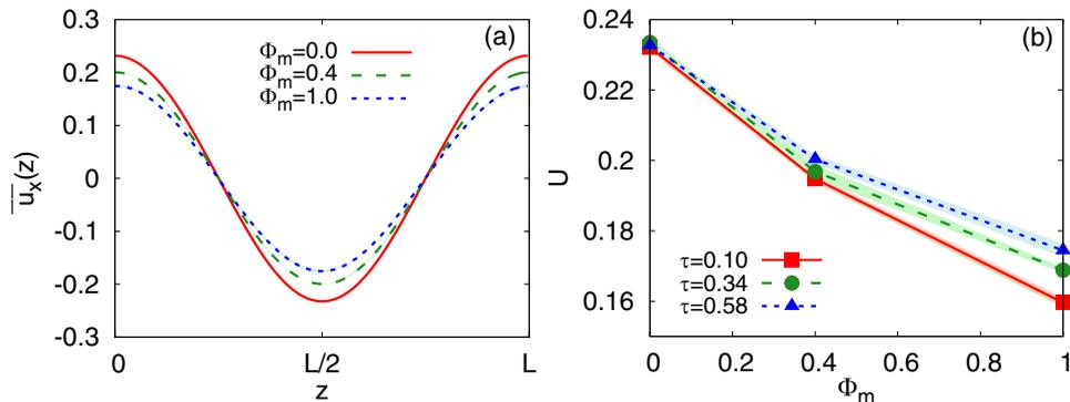
FIG. 2. Averaged profiles and amplitudes of the longitudinal fluid velocity. (a) Mean velocity profile  $\bar{u}_x(z)$  for different mass loading  $\Phi_m = (0.0, 0.4, 1.0)$  and fixed  $\tau = 0.58$ . (b) Amplitude of the mean flow  $U$  as a function of  $\Phi_m$  for different Stokes time as in label.
