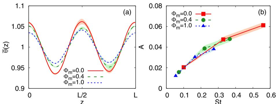
FIG. 5. (a) Mean particle density profile  $\bar{\theta}(z)$  for different values of mass loading  $\Phi_m = (0.0, 0.4, 1.0)$  and fixed Stokes time  $\tau = 0.58$ . (b) Amplitude  $A$  of the spatial modulation of the density profile  $\bar{\theta}(z) = 1 + A \cos(2Kz)$ , as a function of the Stokes number  $St$  for different values of  $\Phi_m$ .
