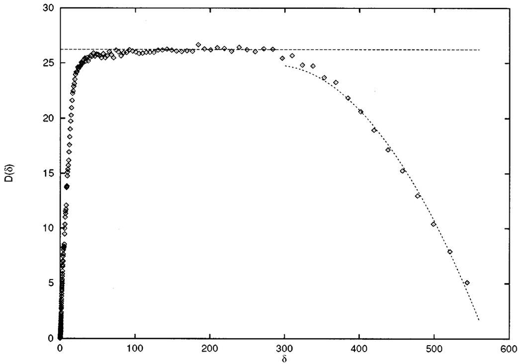
FIG. 4.  $D(\delta)$  vs  $\delta$  for the modified standard map with  $K = 8$ ,  $L = 1000$ , and  $l = 990$ . The series of thresholds is  $\delta_n = \delta_0 r^n$  with  $\delta_0 = 10^{-4}$  and  $r = 2^{1/16}$ . The horizontal line indicates the diffusion coefficient in the limit of the infinite system, the dashed curve represents the saturation regime.
