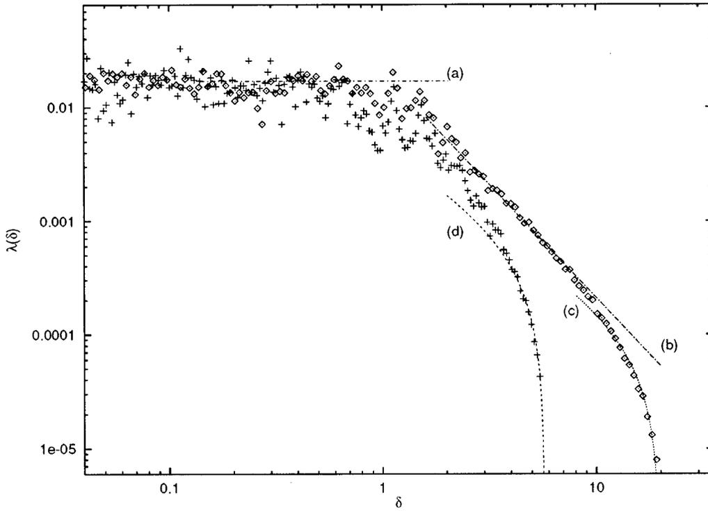
FIG. 3.  $\lambda(\delta)$  vs  $\delta$  for the same model and parameters of Fig. 2, but in a closed domain with 6 (crosses) and 12 (diamonds) convective cells. The lines are respectively: (a) Lyapunov regime with  $\lambda = 0.017$ ; (b) diffusive regime with  $D = 0.021$ ; (c) saturation regime with  $\delta_{\max} = 19.7$ ; and (d) saturation regime with  $\delta_{\max} = 5.7$ .
