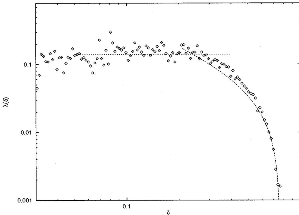
FIG. 6.  $\lambda(\delta)$  vs  $\delta$  for the same model and parameters of Fig. 5. The horizontal line indicates the Lyapunov exponent ( $\lambda=0.14$ ), the dashed curve is the saturation regime with  $\delta_{\max}=0.76$ .
