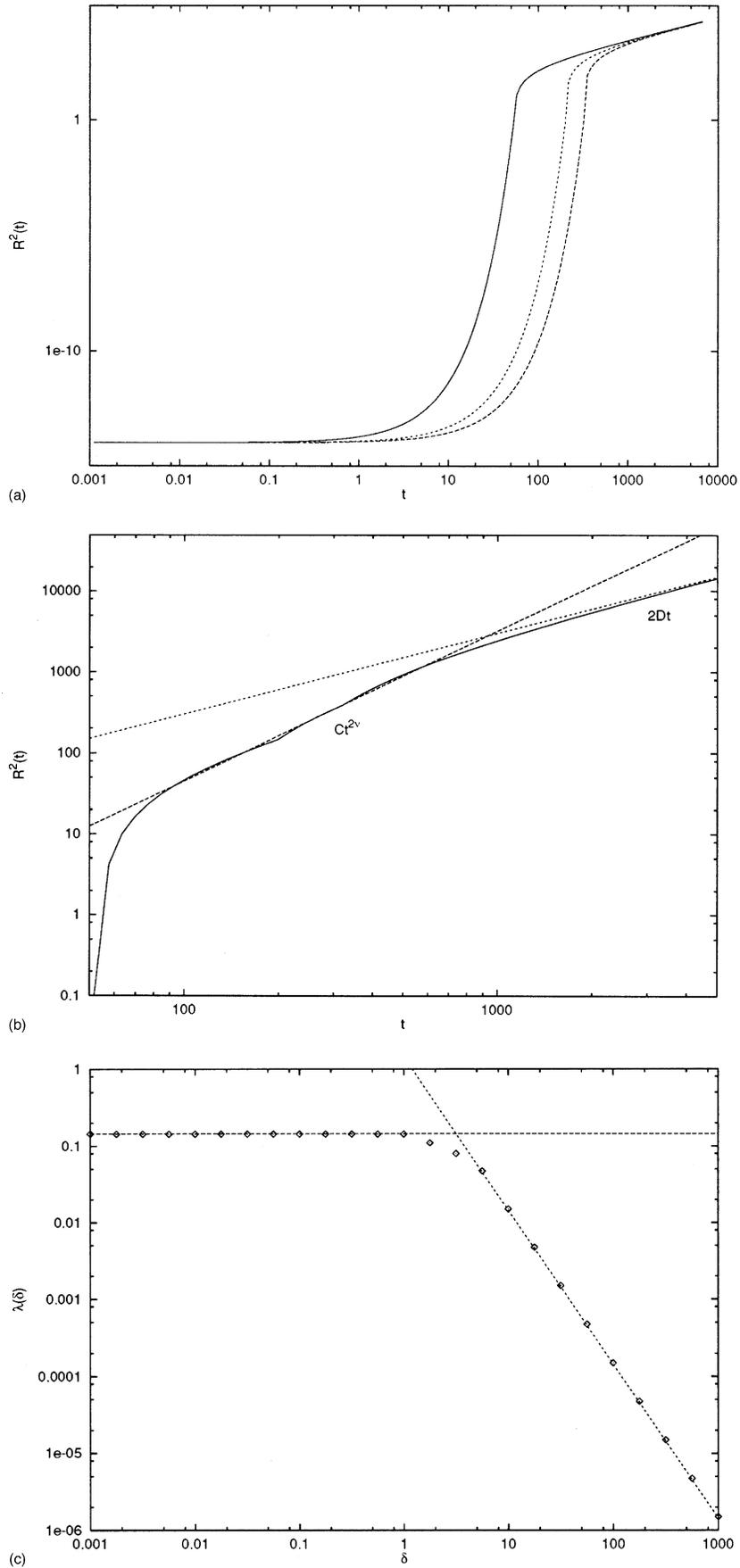
FIG. 1. (a) Three realizations of  $R^2(t)$  as a function of  $t$  built as follows:  $R^2(t) = \delta_0^2 \exp(2\gamma t)$  if  $R^2(t) < 1$  and  $R^2(t) = 2D(t - t_{*})$  with  $\gamma = 0.08, 0.05, 0.3$ , and  $\delta_0 = 10^{-7}$ ,  $D = 1.5$ . (b)  $R^2(t)$  as function of  $t$  averaged on the three realizations shown in (a). The apparent anomalous regime and the diffusive one are shown. (c)  $\lambda(\delta)$  vs  $\delta$ , with Lyapunov and diffusive regimes.
