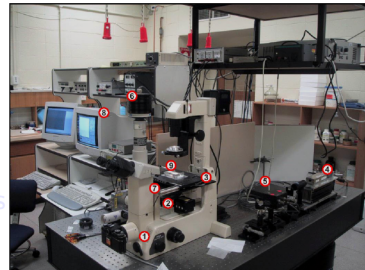
Figure 2.9: This photo was taken in June 2005, after the system was significantly modified. The components in the photo are: (1) Nikon Diaphot 300 inverted microscope, (2) Microscope objectives, (3) Microscope stage, (4) Coherent Compass 4000M Laser, (5) BEOC Laser Stabiliser, (6) MTI IFG CCD Camera, (7) Physik Instrumente Piezo Translator, (8) replacement control computer with custom written Labview software, (9) Sample Cell built in-house.
