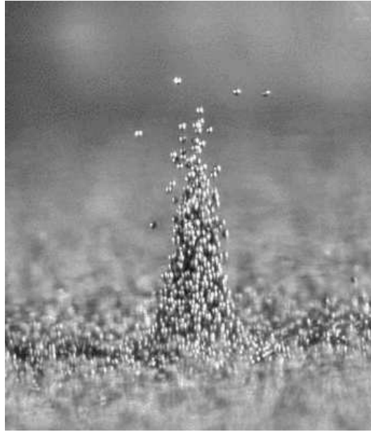
Figure 1.12: The oscillon: a two-dimensional solitary standing wave on the surface of a granular monolayer
