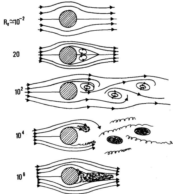
Fig. 5. Schematic pictures of the behaviour of a fluid around a cylinder at different Reynolds numbers.
