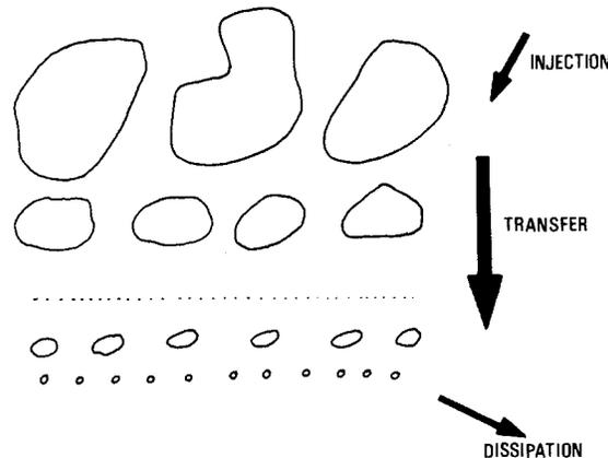
Fig. 6. Scheme of the energy cascade. The reader must think that successive eddies are embedded one within each other.
