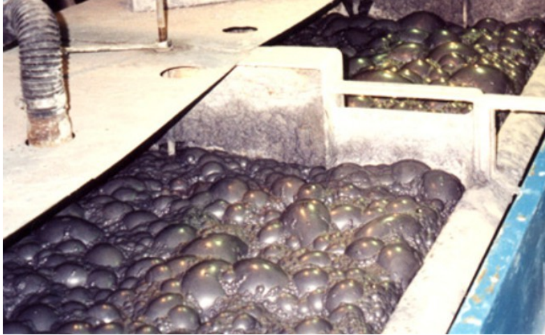
Ore separation (copper extraction by flotation)
